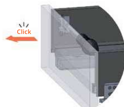
Sgancio frontale Drawer Front Quick Release
